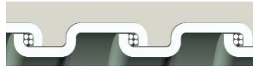
Square-Locked Design with cord packing 3/8" through 1-1/4"
