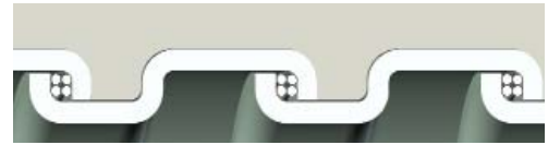
Square-Locked Design with cord packing 3/8" through 1-1/4"
